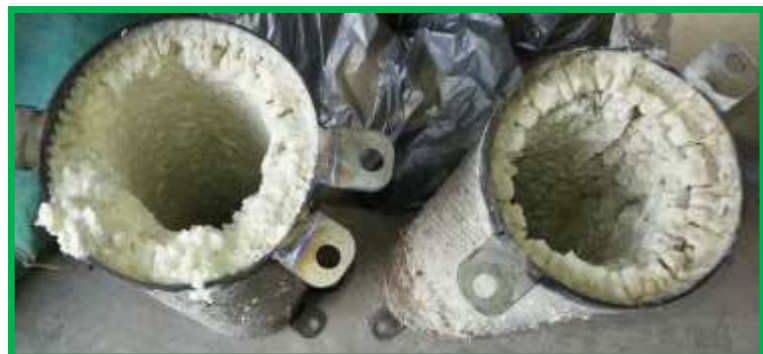
After 2 weeks' operation, ionizer accumulated with scale deposit
