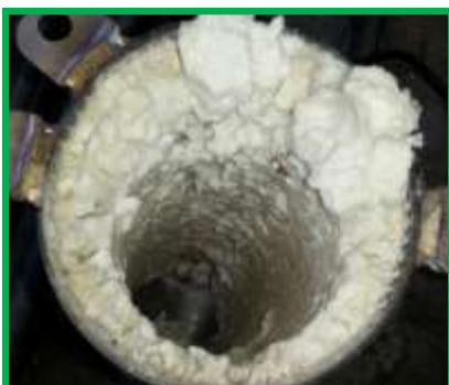
After 2 weeks' operation, ionizer accumulated with scale deposit
